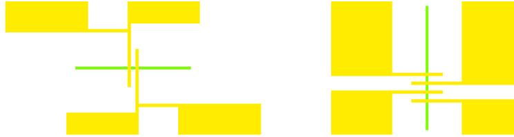
**Figure 3.3:** The design of the easy axis junction (left) and the hard axis junction (right). The green structures represent  $\text{CrO}_2$ , the yellow structures the MoGe-Ni-Ag trilayer.
