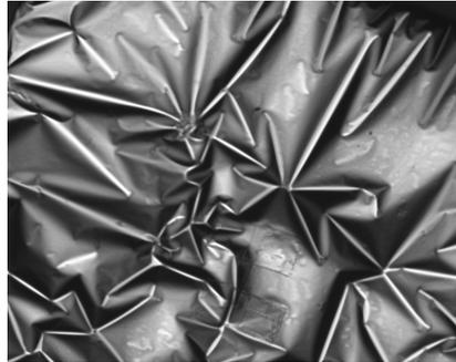
**Figure 3.7:** This figure shows what a sample (BSV8, see section 4.3.1) looks like before lift-off. The PMMA layer underneath the sputtered trilayer has been solved in acetone, that is what causes the folds.
