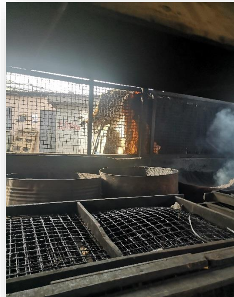
Smoking is conducted within a smoking chamber'. The smoke basins/racks are charred from the smoke residue. In the chamber there are around 8-9 ovens of different makes (Morrison and Chorkor).
