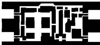
Figure A.3: Mask of the PCB that was designed to hold our double tank circuit. This mask should be mirrored and printed on some tracing paper in order to use it for etching (section 3.5).
