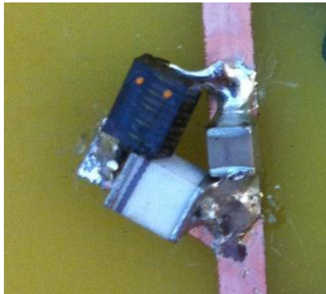
Figure 15: Q-spoiling circuit attached to a main coil with 2 neighbouring coils used in the research project. Here L = 33 nH and C = 5.6 pF
