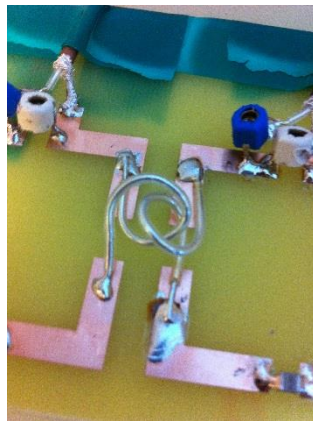
Figure 23: Decoupling circuit consisting of 1 inductor with 1 winding per coil twisted together. The decoupling circuits are made of silver wire.
