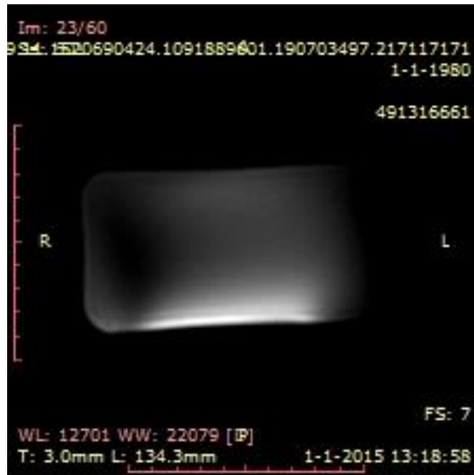
Figure 30: Low tip angle gradient echo image of a phantom bottle filled with a solution of sodium chloride with a concentration of 70 mMOL/L. An array of 2 receive coils was used to acquire the image.
