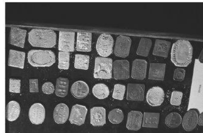
Figure 1. The lead tokens covered with white corrosion and surrounded by white particles are suffering from active corrosion; the other tokens are not.
