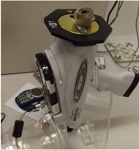
Fig. 7.2: The XRF analysis of the crucibles (24-1-2012).
