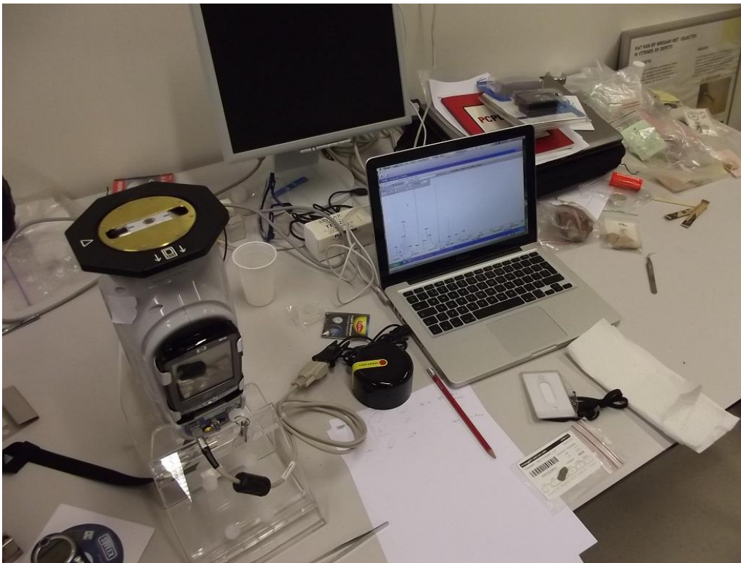
Fig. 7.3: The Bruker Tracer III-S, linked to a MAC laptop. The black cap is placed over the object before the X-rays are fired. Attached to the front of the device is a portable XRF-instrument.
