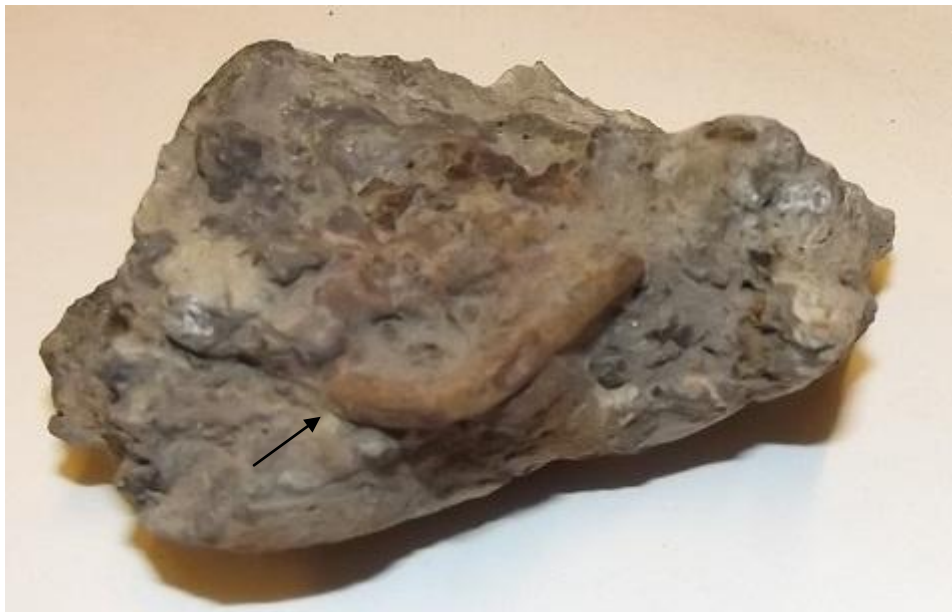
Fig. 2.9 A piece of iron stuck in smithing slag (arrow). Findnumber V00196MXX, trench 8, feature 1 (size ± 63x43x22 mm).
