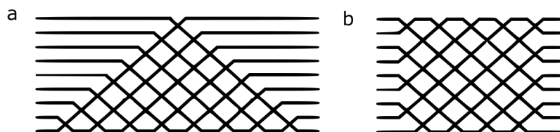
Figure 2.5: a) The design of the interferometer after Reck decomposition. b) The design after Clements decomposition for the same amount of modes. Figure adapted from [18].
