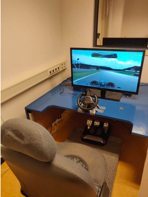
Figure 2. The set-up of the driving simulator used for both the experimental and the control condition. Participants drove (or viewed a recorded video of) 3 laps on the Twin Motegi Course as displayed.
