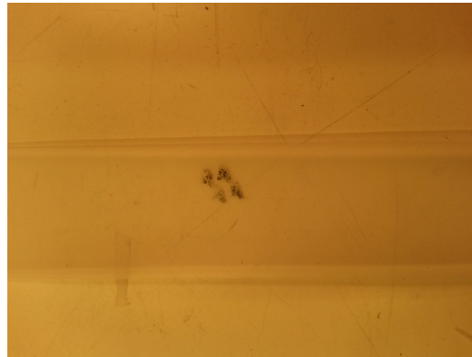
Figure 3.1: A piece of scotch-tape with flakes. Exfoliation has been performed thrice.
