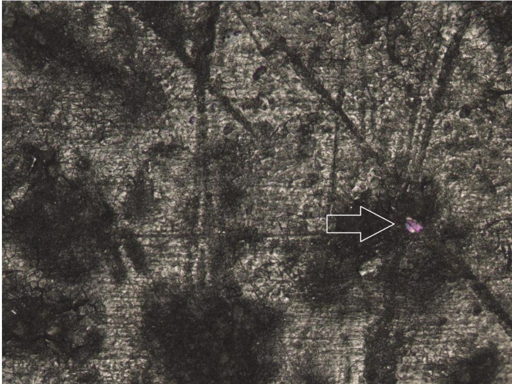
Figure 14 Instance of a mineral inclusion in jet as seen by the author on a 200 X magnification of the surface. This is possibly quartz or zircon.
