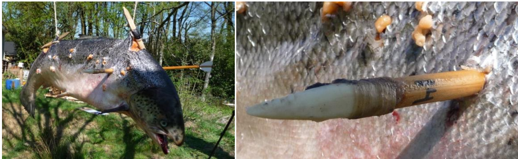
Figure 17: (left) Experimental point 3641 shot for the 12th time, into the back of the salmon with a penetration depth of 20.5cm.
