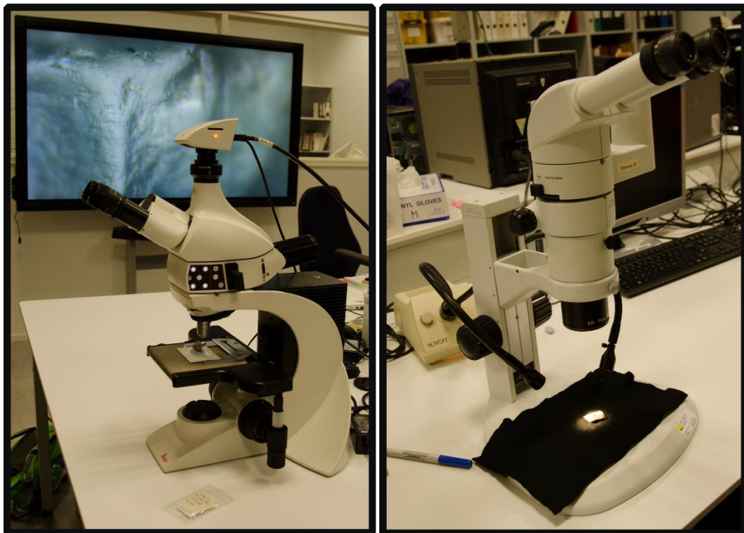
Figure 46: Left Leica® DM1750M microscope with 2.5 Megapixel HD Microscope Camera Leica® MC120 HD camera, right Nikon® SMZ800 stereomicroscope with Schott KL200 light.
