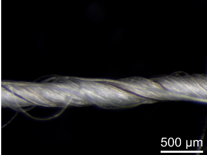
3.5.7 Combed sample 20: combed Shetland fibres, sample bag 7. spun z by Jasmijn Nobelen with spindle whorl VO1694ker in bottom position
