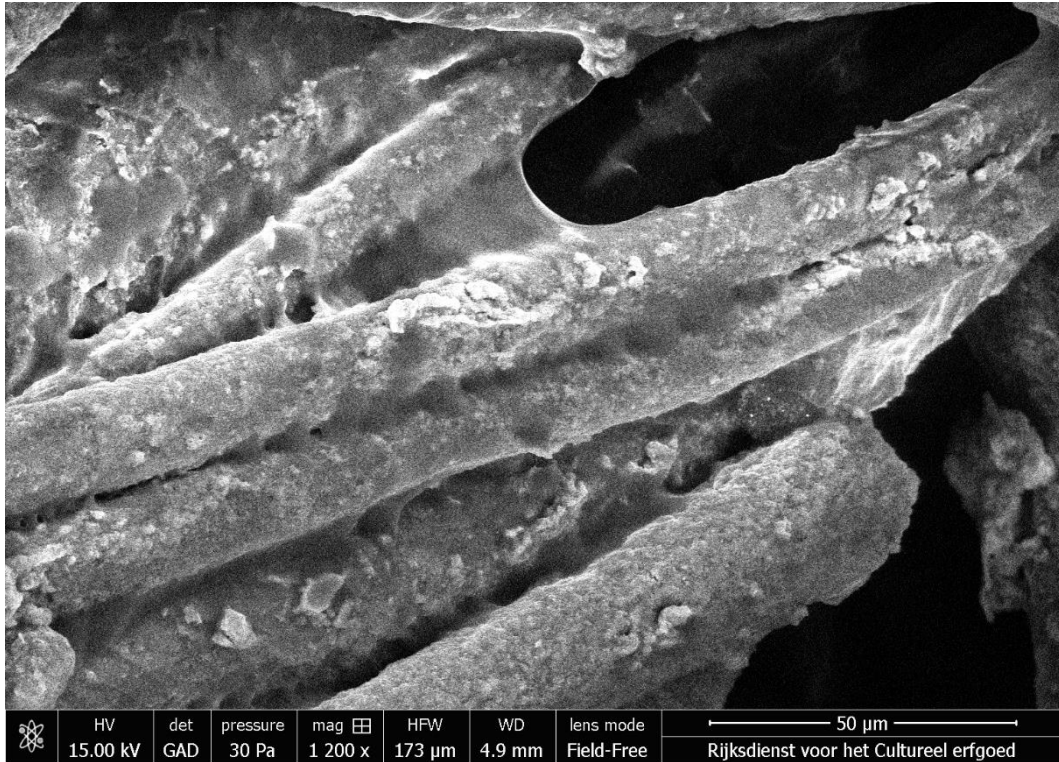
Figure 18 Close-up of the substance covering the fibres of sample Slabroek-70A (possibly the PVAc) (© Cultural Heritage Agency)
