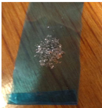
Figure A.6: The Nitto tape with bulk MoS 2 as used for exfoliation
