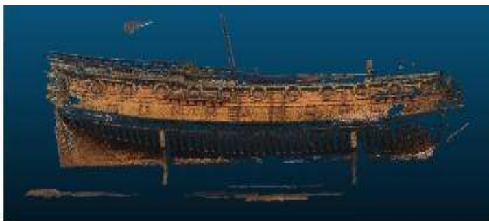
Figure 5.39: The dense point cloud of the ship model using VisualFM ( http://www.usna.edu ).
