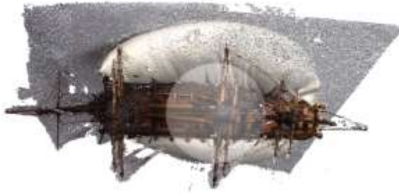
Figure 6.51: The dense point cloud of the top of the model (after the author 2019).
