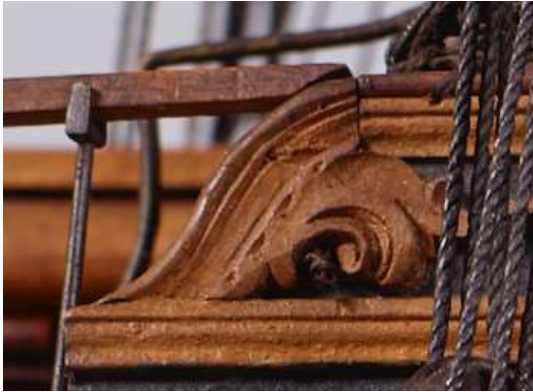
Figure 2.7: The hance dropping from the quarter deck to the waste (after the author 2019).
