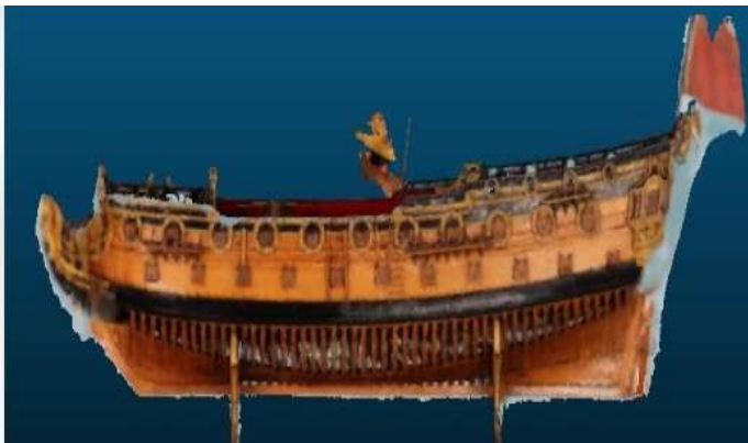
Figure 5.38 : The dense point cloud of the ship model using Agisoft ( http://www.usna.edu ).
