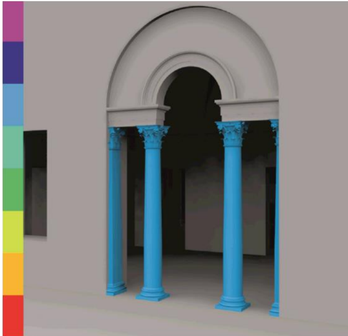
Figure 8: Project for twin columns from Palladio in which a color code is used to encode the uncertainty within the columns (Apollonio 2016, 191).
