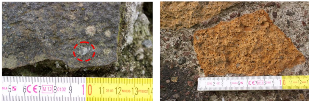
Figure 23: One leucitite crystal in the dark material on the left is highlighted by a red-dashed circle. One exemplary tuff block is located on the right (Brunke 2017).
