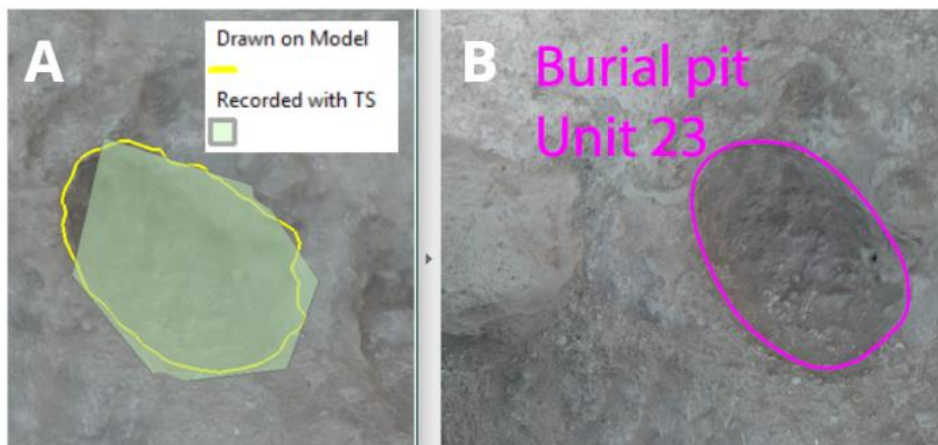
Figure 6.3: Difference in geometric accuracy between recording pit unit BX13_24 using a total station and by drawing the contour directly atop the photogrammetry model within ArcScene. (A) Comparison of different recording strategies; (B) annotated plan drawing (figure by author).
