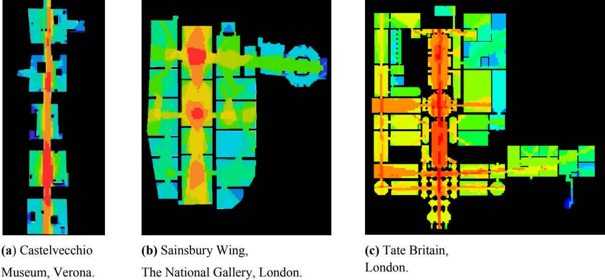
Fig.6. Examples of shallow core: warm colours represent areas of high visual integration; cold colours show areas that are less visually integrated. (Not to scale.)
