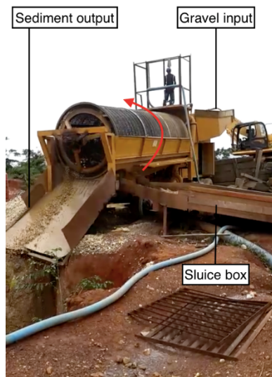
Fig 4. Tromel at Key Empire’s washing station (Picture by Emmanuel)
