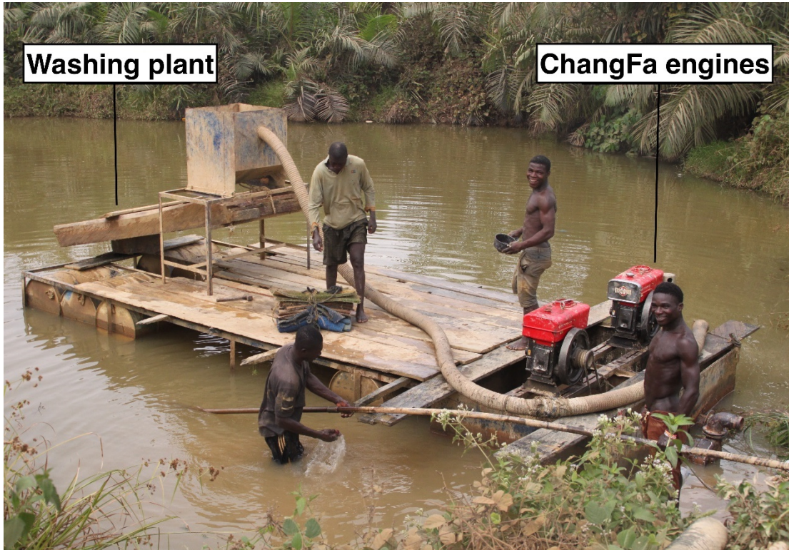
Fig. 2.2 A dredge in one of Key Empire's old pits (picture by author)
