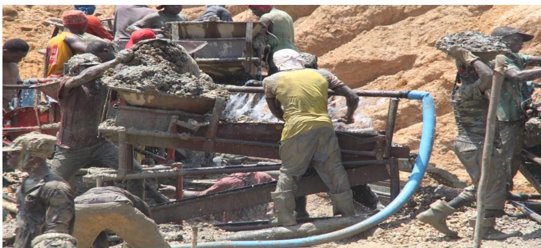
Fig. 1. Suagum with traditional washing plant on the concession of ATK-mining (picture by author)
