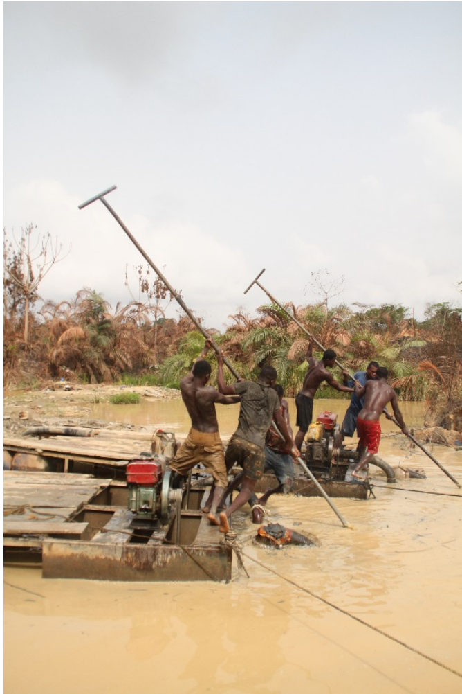
Fig. 2.1 Two dredges in one of Key Empire's old pits while loosening the bottom of the pit and extracting the gravel (picture by author)
