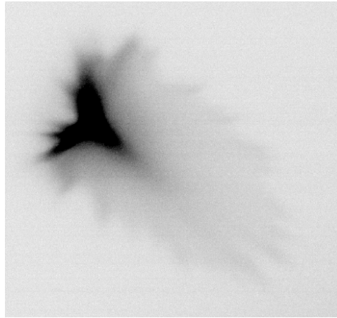
Figure 4.3: Image of the electron beam, directly focused on the detector with the prisms turned off. Contrast is inverted for clarity, the darkest spot has the highest intensity.
