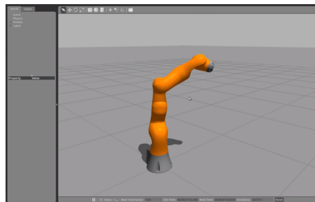
Figure 5.11: Screenshot of the KUKA robot model in the Gazebo environment.
