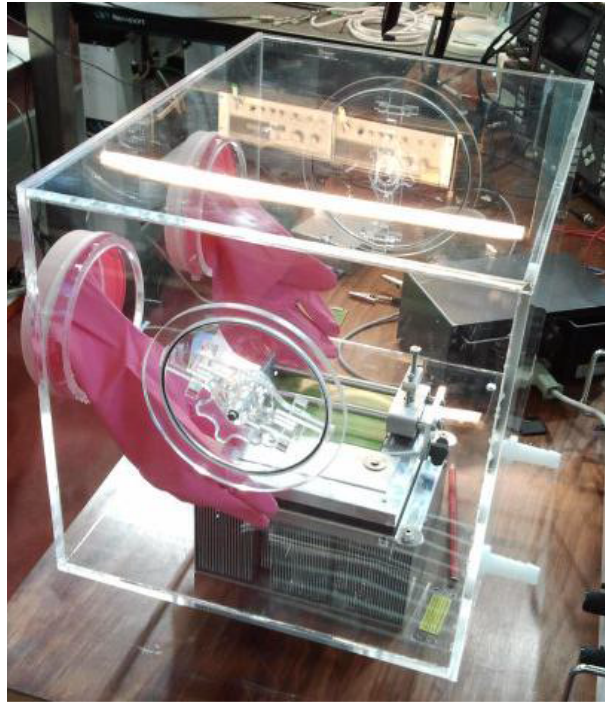
Figure 3.1: The old set-up. The box surrounding the experiment is to prevent water vapor in the air to enter the set-up and contaminate it with ice.
