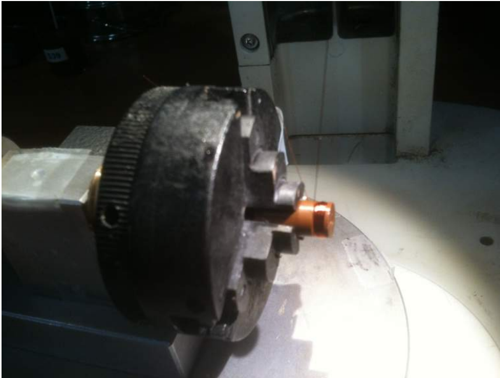
Figure 3.5: The holder in the rotating device. One end of the wire is taped to the rotator and the other is held with tension from the wire coil.
