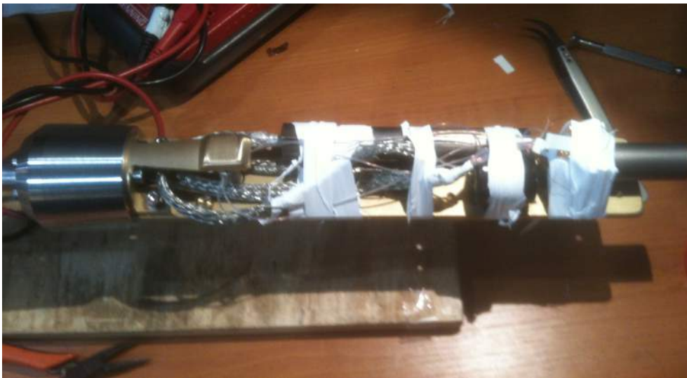
Figure 3.18: The experiment taped together with teflon tape. This way everything stays tight together.
