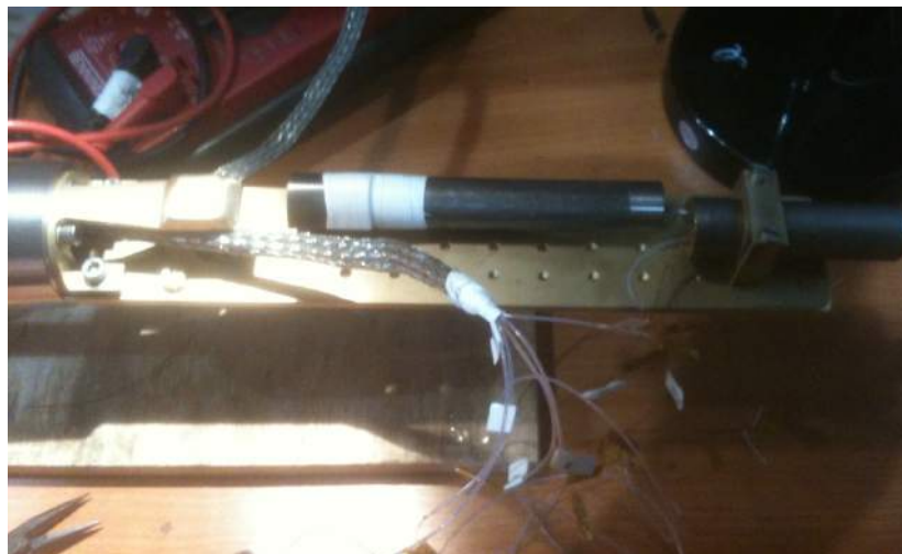
Figure 3.17: The elliptical coils are put some notches back to make room for the SQUID.
