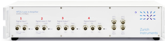
Figure A.1: The lock-in of our set-up. Parts 1 en 2 are inputs, parts 3 en 4 transfer output signals.
