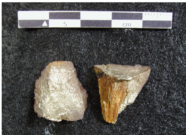
Figure 3.9. Photograph of sulphuric iron nodule fragments exhibiting unweathered (left) and weathered (right) fracture surfaces.
