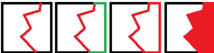
Fig. 10: making polylines into areas in four steps (left to right)
