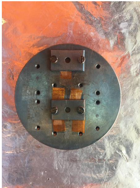
Figure 4.5: The used sample holder of the TRE. The contours clearly show the placement of previous samples.
