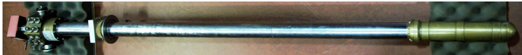
Figure 3.2: The dipstick, horizontally positioned. At the bottom (right) the sample is placed in the sample holder and at the top (left) all electrical wiring is connected to external ports.
