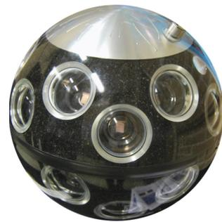
**Figure 2.2:** A Digital Optical Module (DOM) housing 31 photomultiplier tubes (PMTs)
