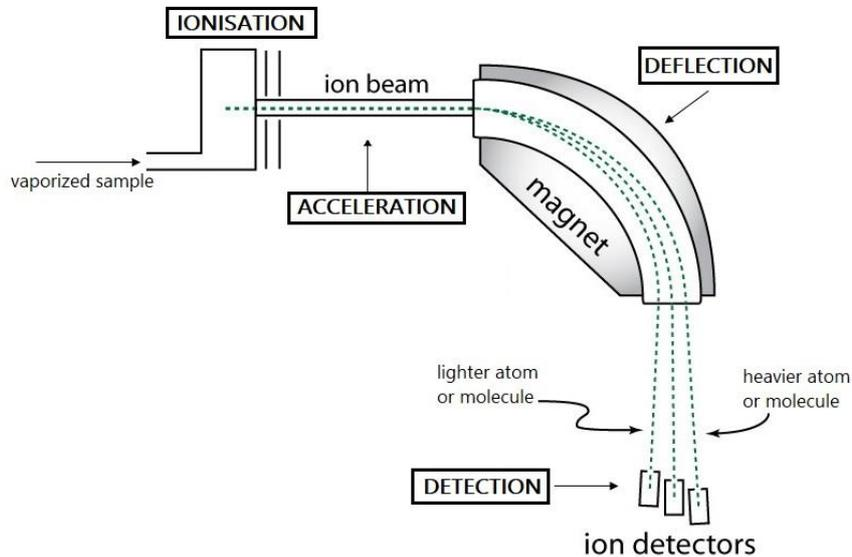
Figure 1 – A Mass Spectrometry Schematic: the arrangement of the basic components of a mass spectrometer. Figure taken from Sercmedia (<https://serc.carleton.edu/download/images/9094/massspecschematic.jpg>) edited by the author.
