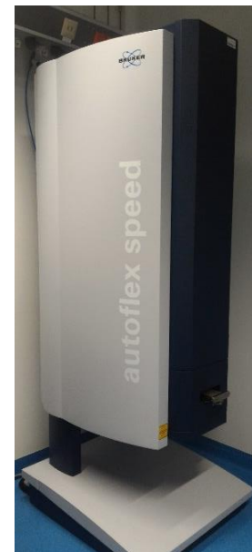
Figure 14 The autoflex LRF MALDI-TOF mass spectrometer used in this research, picture from Virginie Sinet-Mathiot.
