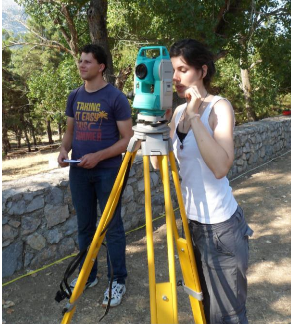
Figure 2.4: Working with the Total Station. The device is set up exactly level on a tripod, and aimed at the reflective prism. (Photo: Jordy Aal 2011)
