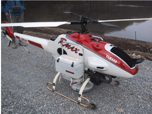
Figure 30: A Yamaha R-Max remote-controlled survey helicopter or UAV outfitted with a camera and GPS tracking system (Everaerts 2008)
