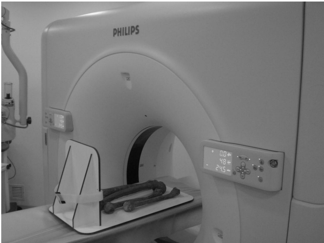
Figure B.1. Limb bones placed in the CT scanner on a custom made board.
