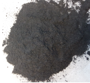
Fig. 3.1 PG powder. The diameter of the particles is 44\text{ }\mu\text{m} .
