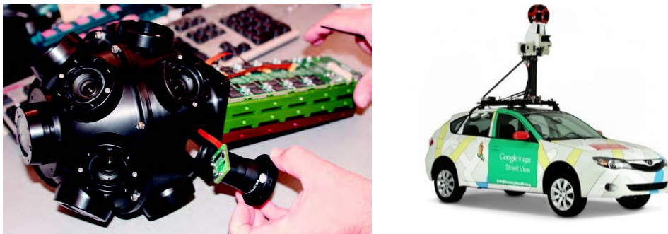
Figures 0.1 and 0.2 A rosette camera set with fifteen cameras is installed on all Street View vehicles.
