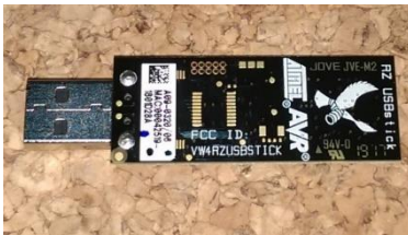
Figure 16: Capturing ZigBee network traffic with the ATMELE RZUSBSTICK, Killerbee software and WireShark.
