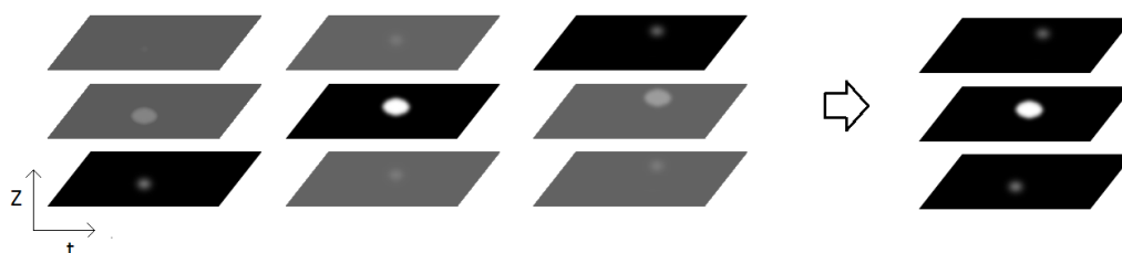
Figure 2.18: Movement between slices. The three stacks on the left show the actual point spread function of a particle across three slices, at three successive points in time. The particle is centred on the middle slices and is moving in the XY plane. The darkened slices are those actually acquired up by the microscope, due to its lag. The subsequent distorted Gaussian can be seen in the stack produced on the right.
