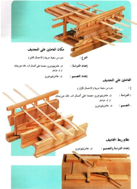
Figure 9 Placement of oarsmen and system of attachment of oars (Hatzitheodorou 2004, 15)
