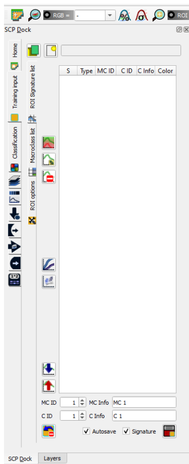
Figure xix: Screenshot of the SCP dock with the training input tab open, ready to enter Regions Of Interest (ROI) for different classes.
