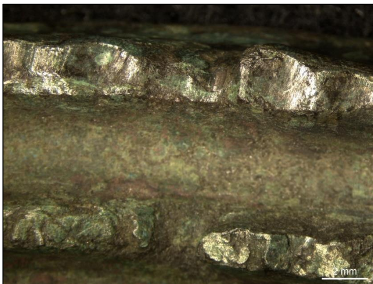
Figure 5.14: detail of the transversal striations located on the ribs and the deformations of E2010/Ede
