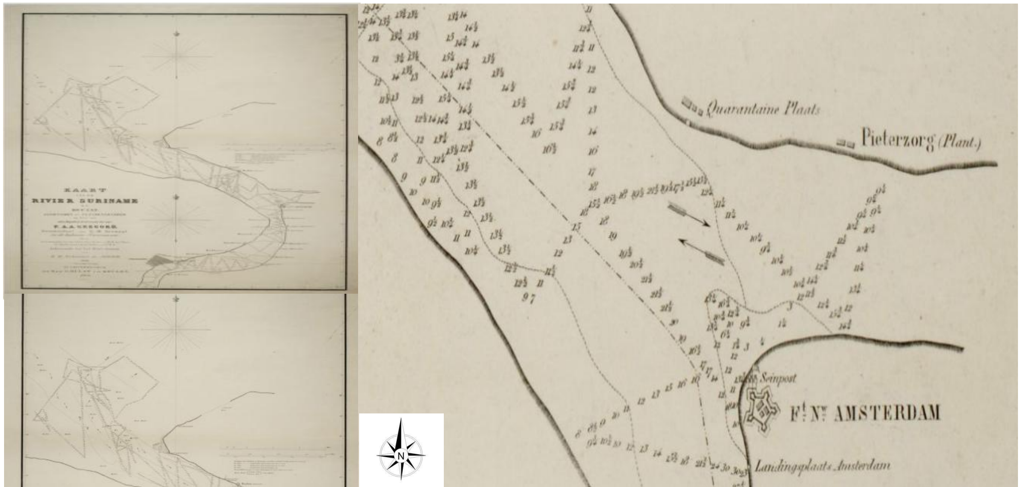
Figure 13. Nautical map showing the projected fairway larger ships would take. This map is calculated in Amsterdam feet (at 0.2831 m) from the mouth of the Suriname River to Paramaribo, reduced to low tidewater. This revision dates from 1869. The original handwriting card, which was compiled on board the naval vessel Z.M. Adder in 1860, is kept in the Library of the former Ministry of Colonies ( http://dpc.uba.uva.nl )
