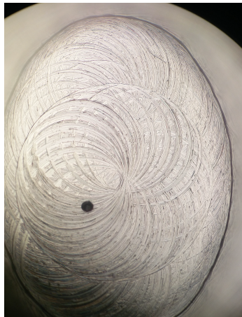
Figure 3.3: Optical microscopy picture of the inside the lead trap with the magnetic particle is laying at the bottom. This is an elliptical shaped trap, which will be used for future experiments. The traps used in our samples are circular.
