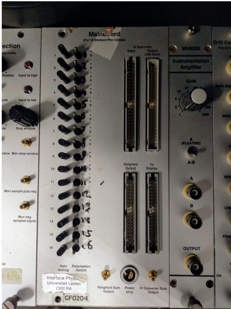
Figure 3.4: Summing module. The signal from the 16 photodiodes goes into "Input". When the gain settings and polarisation switch are tuned accordingly, the weighted sum output is the deflection signal.
