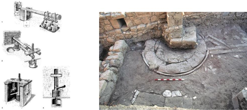
Figure 15: a. Four kind of presses. 1. Lever and weights press; 2. Lever and screw press; 3. Direct screw press with grooved stone piers frame; 4. Direct screw press with a hewn cross-shaped frame (after Taxel 2013,362)
