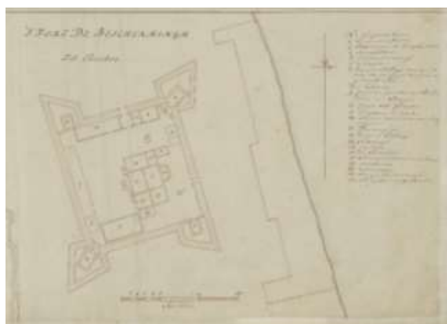
Figure 3.1. Plan of Fort Bescherming in Cirebon. The different shapes of the bastions are narrated by Dagh-Register van Het Casteel Batavia , 8th March 1686 as “two whole-shaped bastions and two half-shaped bastions.” Source: Unknown, Platte Grond van 't Fort de Beschermingh Tot Cheribon Plan van de Werken Tusschen de Spruit Sikaro Ende Groote Rivier van Indermajo De Spruit Sinkaro by Indermajo, van de Negory Diapok Passer Tot de Groote Rivier van Indermajo , Kaartcollectie Buitenland Leupe (Cheribon, Indermajo, Seventeenth Century).
