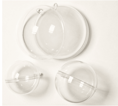
Figure 3.1: The polystyrene ball lens in some different sizes [16].
