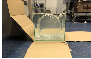
Figure 3.10: The polystyrene ball lens, here filled with sugar solution, inside the aquarium.
