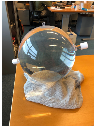
Figure 3.6: The glued-together polystyrene ball lens, filled with water.
