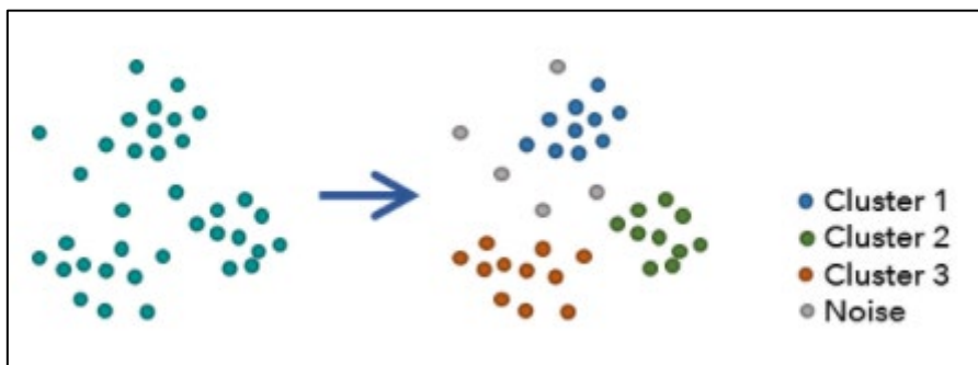
Figure 5.13 Example of how the Density Cluster Analysis tool works. From Esri https://pro.arcgis.com/en/pro-app/tool-reference/spatial-statistics/densitybasedclustering.htm , accessed 24 October 2020.
