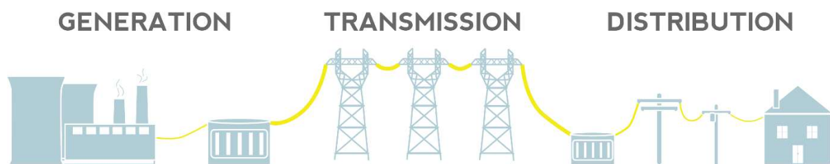
Figure 1: Schematic of a traditional, centralised, unidirectional power grid (IER, 2014).
