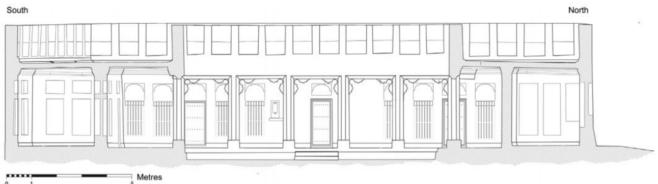
Figure 7. East facing section showing how liwan were erected in Radwani House, (Carter and Eddisford 2017, 85).
